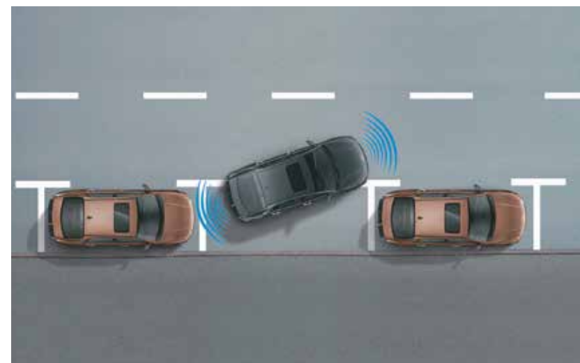
Parking assist (front & rear parking sensors and rear camera with dynamic guidelines)
